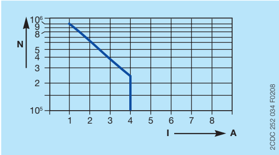
Contact lifetime /switching cycles N 220 V 50 Hz AC1, 360 cycles/h
